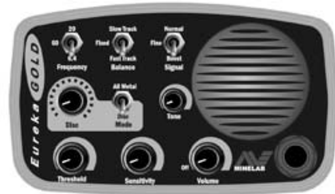
Figure 12 - The Eureka Gold Control Panel
